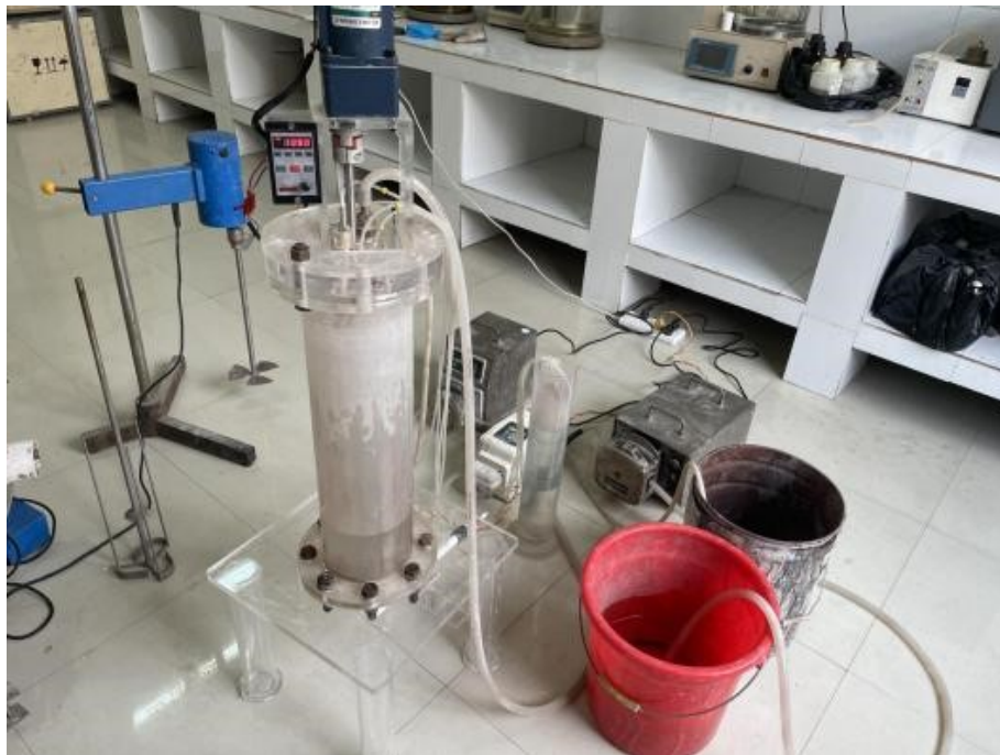
Figure 3. Small-scale continuous dynamic settling experiments.
